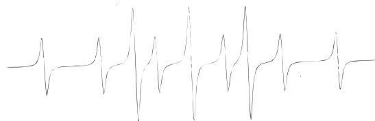
Figure 4. (a) EPR spectrum of spin adduct 12 formed by photolysis of a benzene solution of ethyl iododifluoroacetate in the presence of bis(tributyltin) and NNP at room temperature (microwave power, 5mW; modulation frequency, 100 kHz; modulation amplitude, 0.5). (b) Computer simulation of (a) using the parameters given in Table 4.
